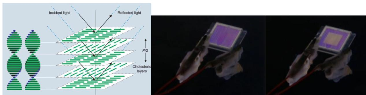
Figure 1: Responsive polymer coatings can reflect daylight in varying wavelength
