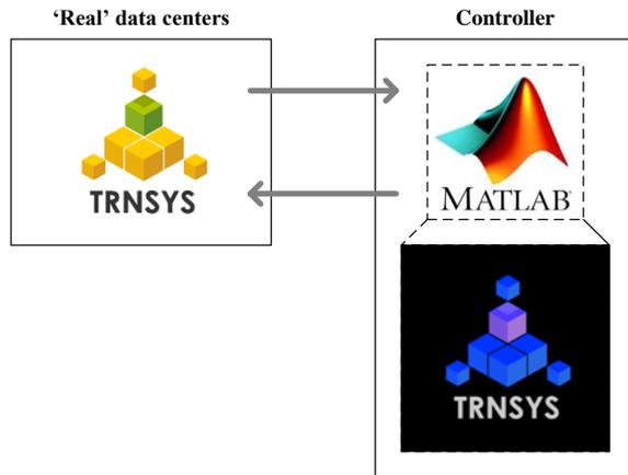
Figure 2: Schematic representation of the test environment consisting of the ‘real’ DC model (TRNSYS) and the controller (Matlab) during simulation run-time. The reference models resides inside the controller; communication inside the controller is based on Matlab scripts.
