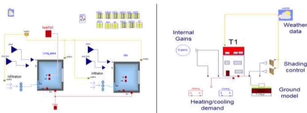
Figure 2 - Model structure in Modelica. Bottom layer (left) and top layer (right). Dark blue lines refer to controls (internal gains and shading control), light blue to fluids (infiltration), red lines to heat transfer (W) and yellow lines to weather related data.
