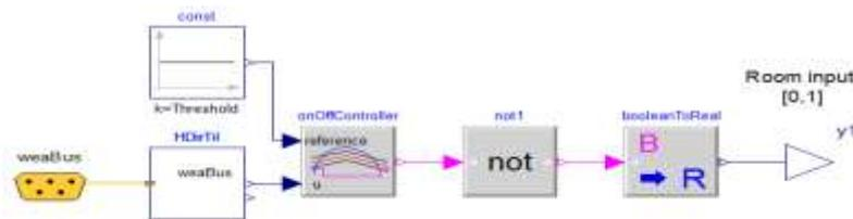
Figure 7 - Implementation of an automatic blinds system for shading control.
