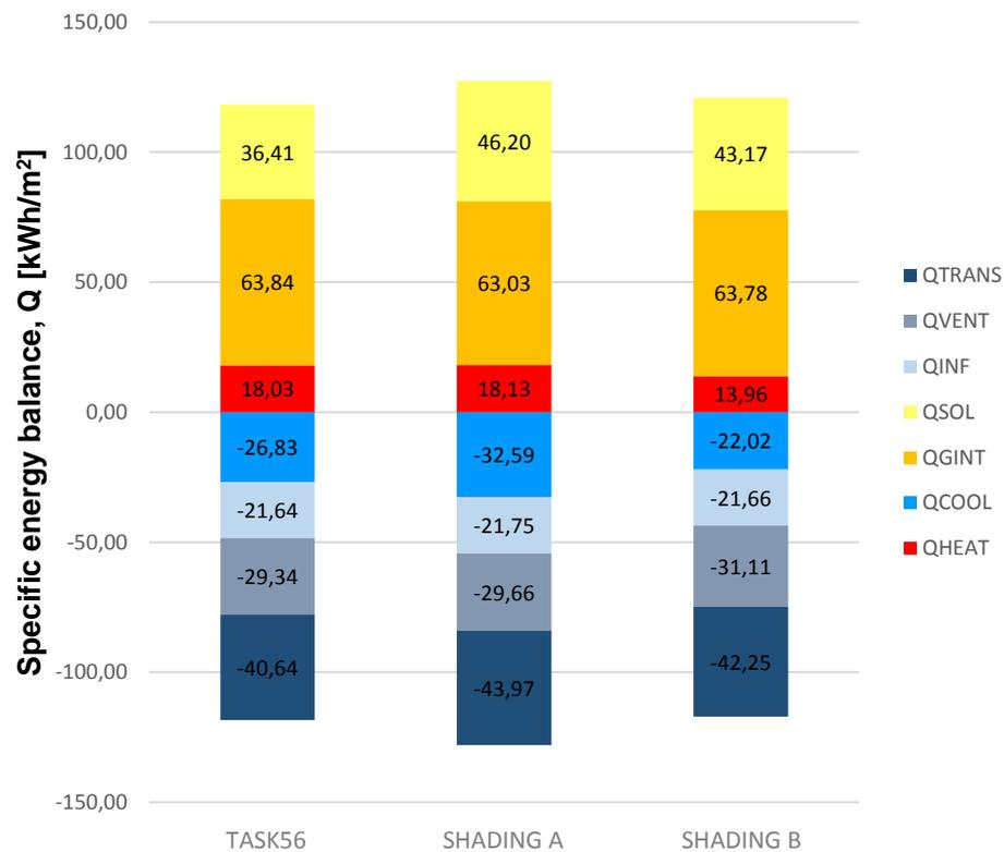
Figure 5. Energy balance comparison between shading systems.
