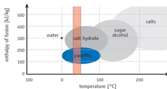
**Figure 2 – Classes of materials that can be used as PCM and their typical range of phase change temperature and melting enthalpy.**
