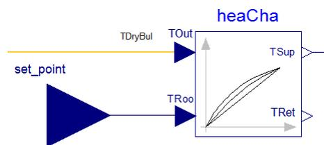
**Figure 6 – *heaCha* - Block used to compute the ideal supply and return temperatures for the heating system.**
