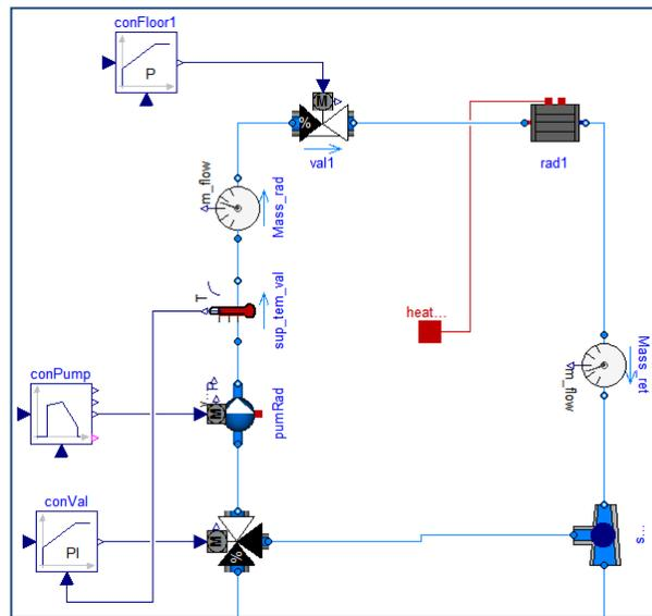
**Figure 5 - Radiator loop model.**
