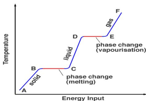
**Figure 1 – Temperature as function of Energy stored in a PCM (B->C)**
