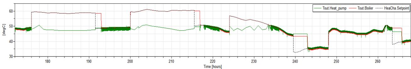
Figure 8 - Temperature of the radiator supply water, for four winter typical days.
