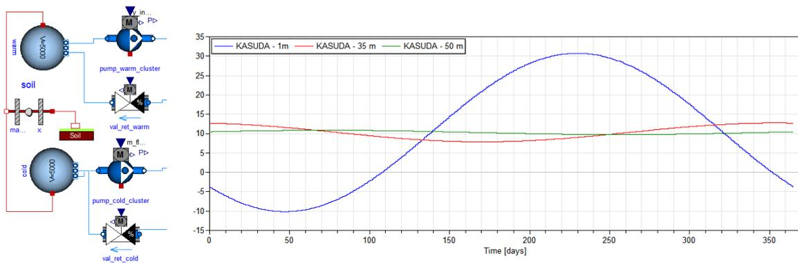
**Figure 10 - (left): ATES model; (right) - Temperature of the soil as function of the depth, using the Kusuda Function.**
