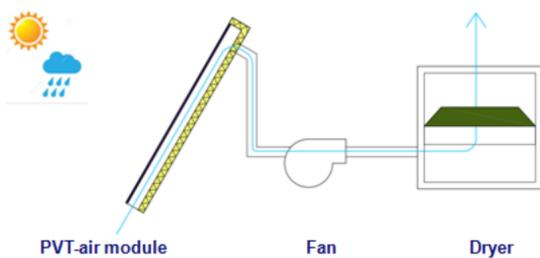
Fig. 3: PVT – air drying system
