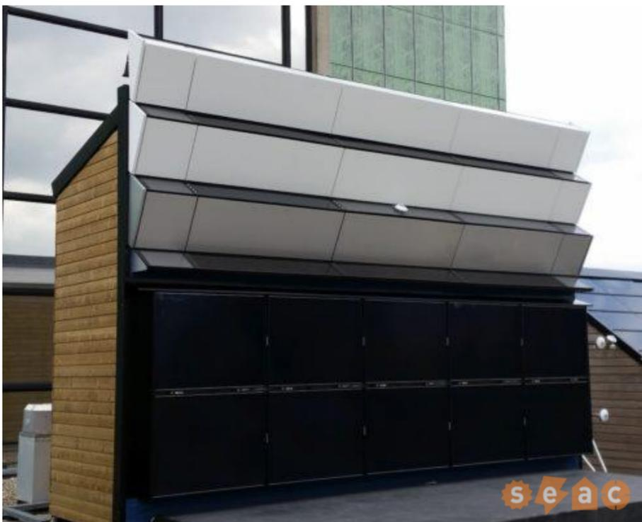
Fig. 1.: BIPV measurement facility at SolarBEAT measurement station
