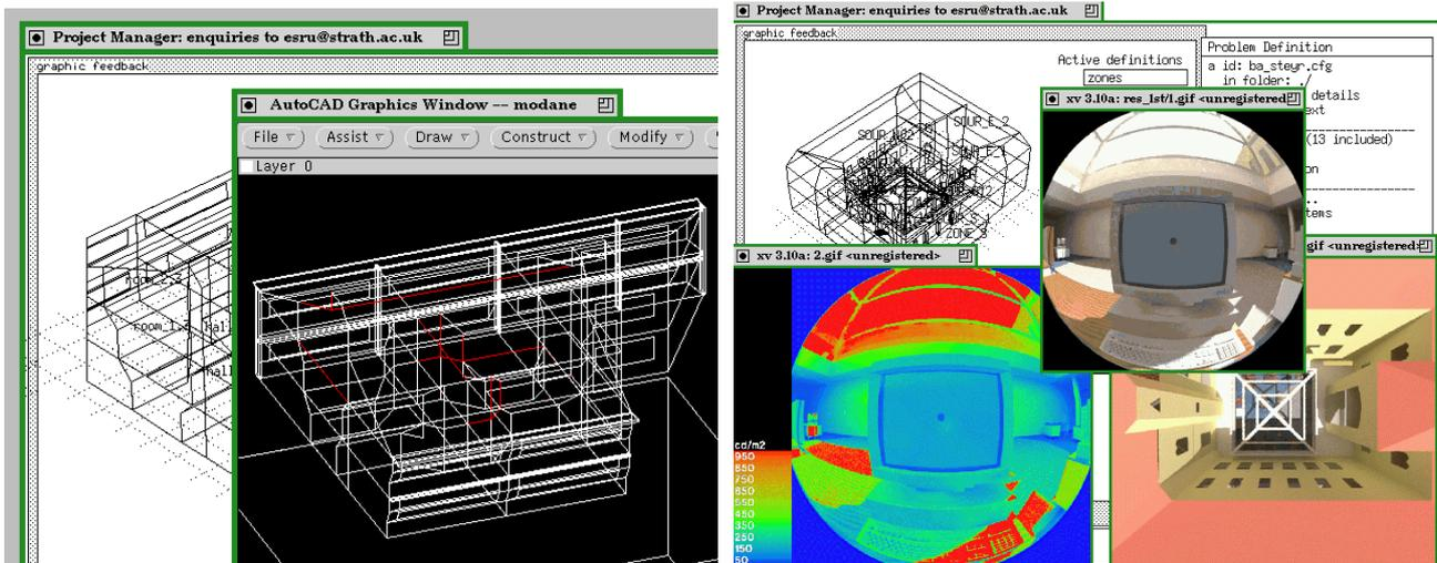
Figure 2 Defining problem geometry using AutoCad (left) and using RADIANCE to quantify luminance for a visual comfort/impact assessment or illuminance as input to a lighting controller (right).
