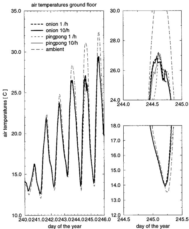
**Figure 5** Simulation results for ground floor air temperatures starting with day 241 and ending with day 246 of a reference year. Frames on the right show selected results in more detail. Temperatures in °C; to obtain °F multiply by 1.8 and add 32.
