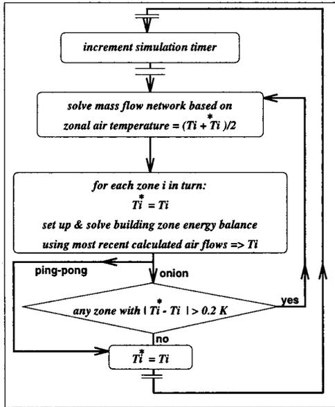
**Figure 2** Schematic flow diagram showing the implementation of a coupled (“onion”) and decoupled (“ping-pong”) solution method for heat and air flow.
