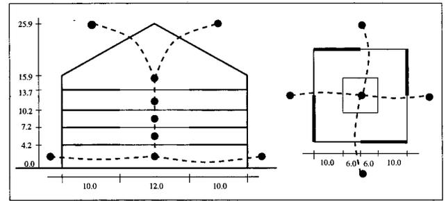
**Figure 3** Cross-section and plan of atrium with air flow network. Dimensions in m; to obtain ft, divide by 0.3048.
