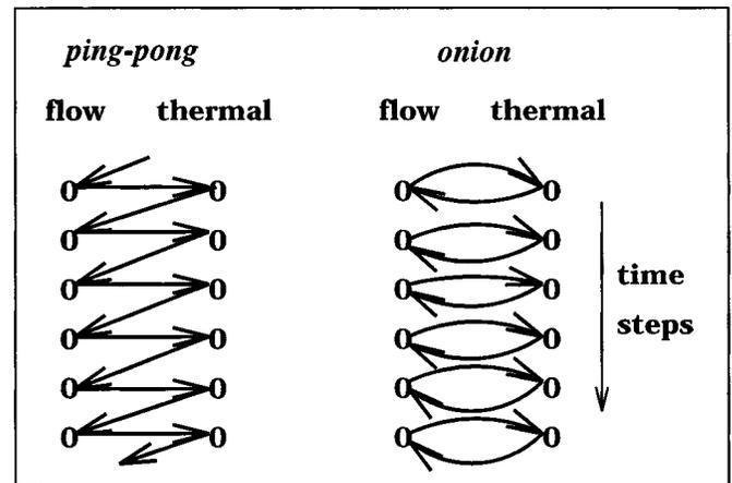
Figure 1 Schematic representation of a decoupled non-iterative (ping-pong) vs. a coupled iterative (onion) approach.
