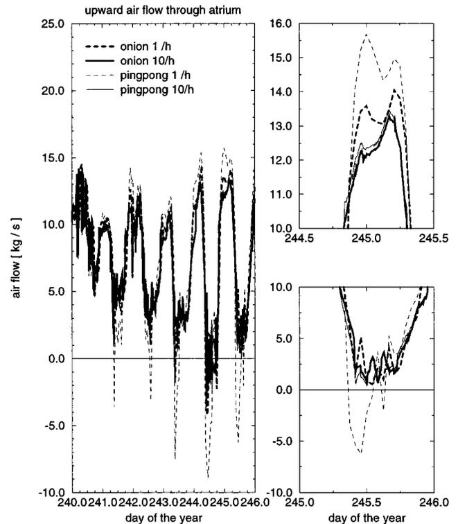
**Figure 4** Simulation results for vertical air flow through atrium starting with day 241 and ending with day 246 of a reference year. Frames on the right show selected results in more detail. Flow rate in kg/s; to obtain lb/min divide by 0.00756.
