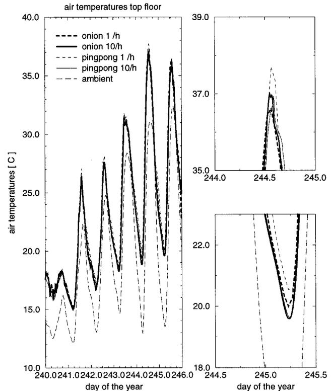
**Figure 6** Simulation results for top floor air temperatures starting with day 241 and ending with day 246 of a reference year. Frames on the right show selected results in more detail. Temperatures in °C; to obtain °F multiply by 1.8 and add 32.
