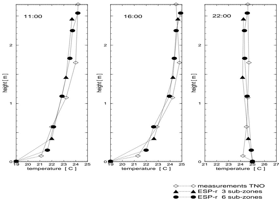
Figure 3 Vertical air temperature gradients for different times during 8 August 1988
