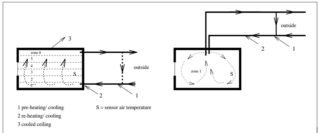
Figure 2 Modelling displacement ventilation and mixing system
