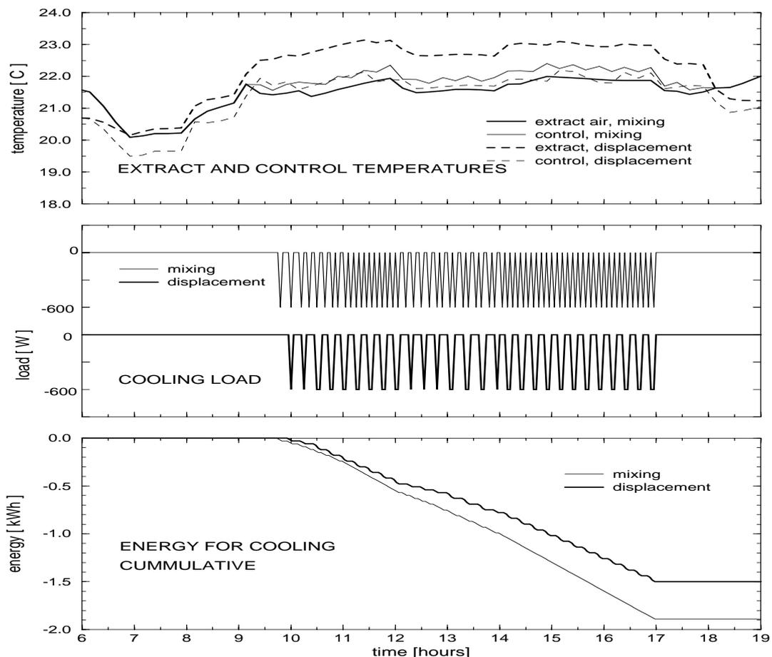
Figure 4 Temperatures, loads and energy consumption in case of cooling mode (for 25 August of a reference year)
