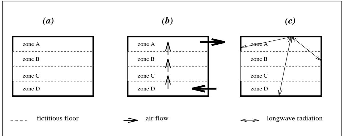
Figure 1 Dividing a zone in stacked sub-zones separated by fictitious floors
