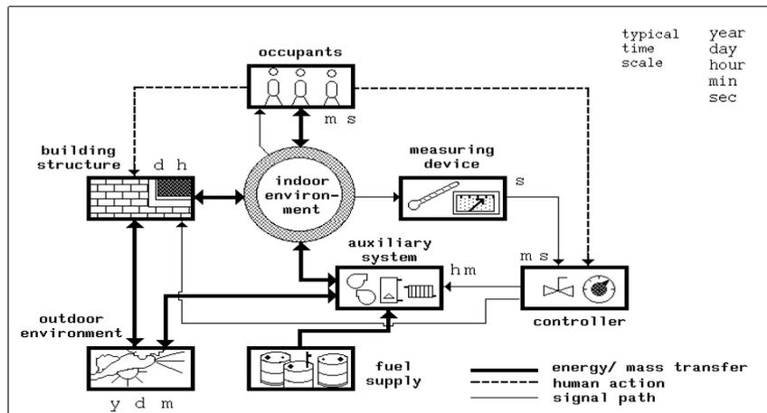
Figure 1 Diagrammatic representation of building and plant
