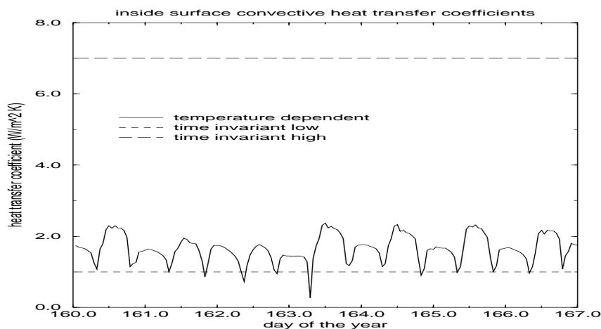
Figure 3 Inside surface convective heat transfer coefficients; fixed and predicted on the basis of surface temperature
