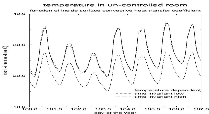
Figure 4 Predicted inside air temperature using temperature dependent respectively independent inside surface convective heat transfer coefficients
