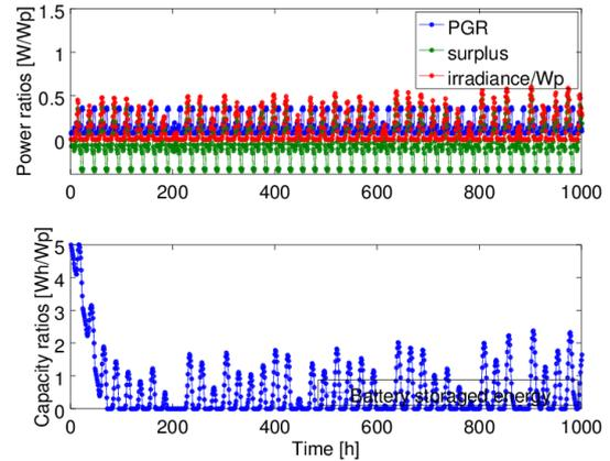
Figure 4. Example of simulation for Murcia with a PGR of 0.15W/Wp, a profile 2 and a storage of 5Wh/Wp during 1000 hours.
