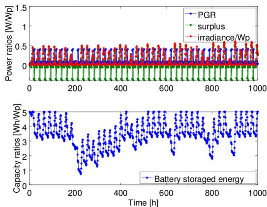
Figure 3. Example of simulation for Murcia with a PGR of 0.08W/Wp, a profile 3 and a storage of 5Wh/Wp during 1000 hours.
