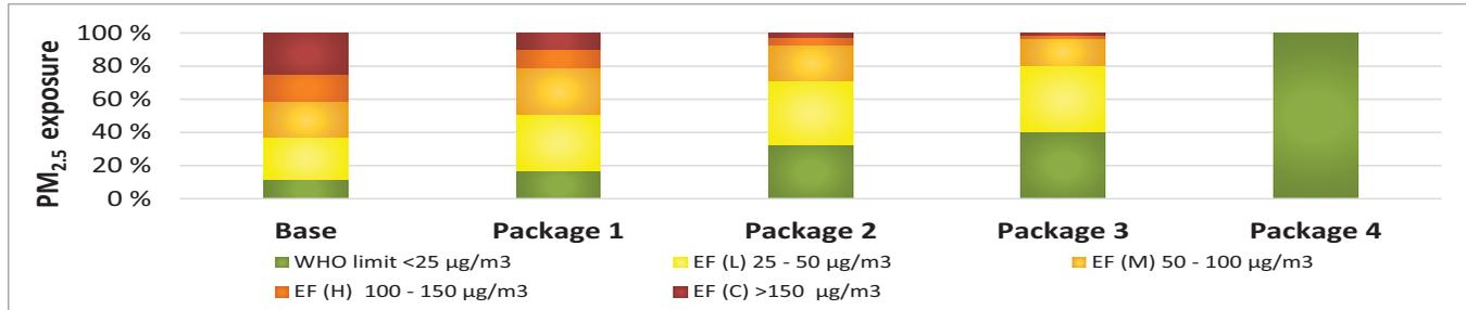
Figure 8: Annual mean indoor PM<sub>2.5</sub> exposure categorized in exceedance factor (EF) hours - Low (L), Moderate (M), High (H), and Critical (C) - and hours underneath daily WHO limit, over in total 1890 occupancy hours
