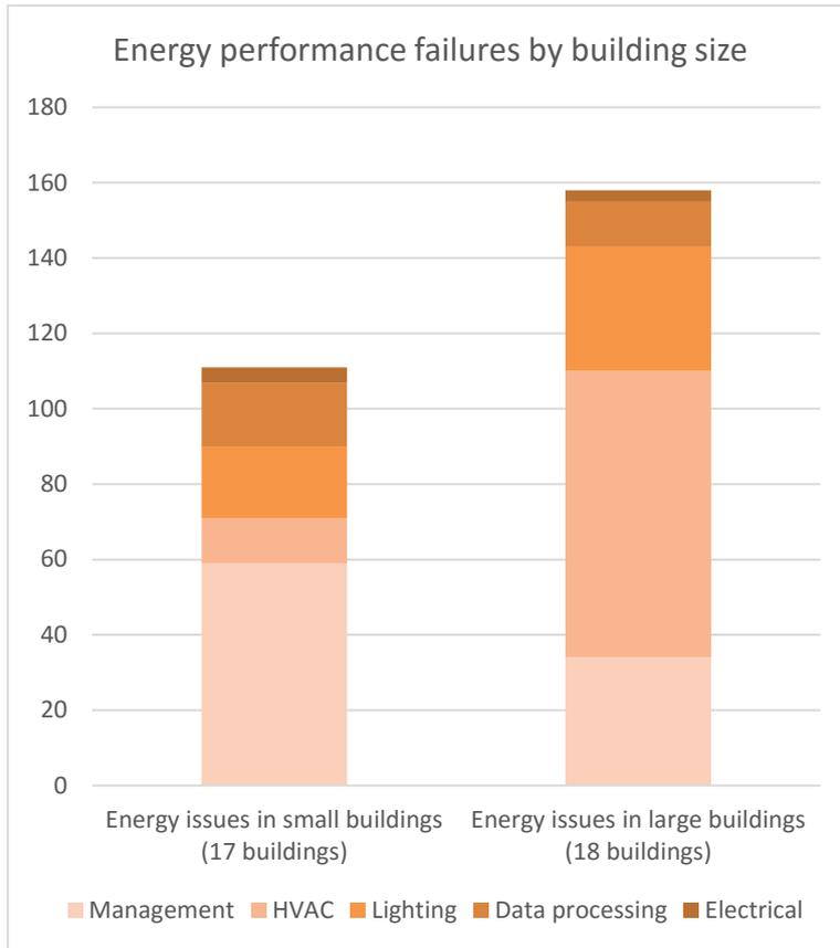
Figure 2 - Number of building energy performance failures encountered in large and small buildings
