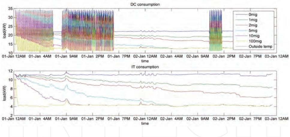
Figure 12. Power consumption with different migration limits over 48-h horizon.
