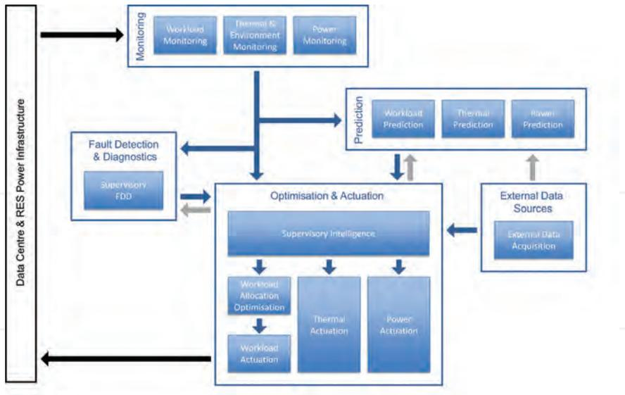
Figure 3. Information flow (simplified) for coordinating workload, thermal and power management [14].
