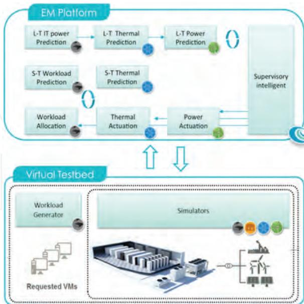
Figure 11. Interaction between EM platform GENiC components and virtual DC test-bed.
