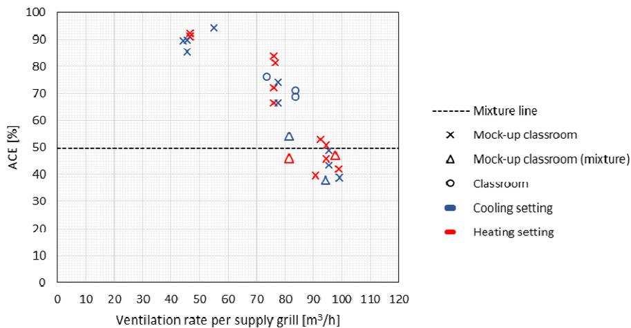
Figure 3. Air change efficiency based on the age of air measured at three positions, at 1.1 m height, in the room. Results from both the mock-up and the real classroom are included.
