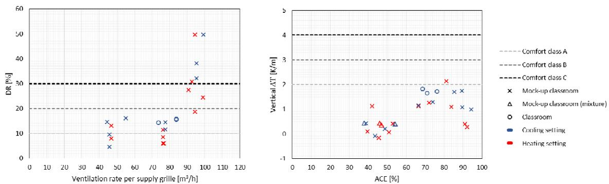
Figure 4. Draught rate as function of the supply flow rate per supply grille (left). Maximal vertical temperature difference as function of the ACE (right). Both graphs present results for the mock-up and the real classroom.
