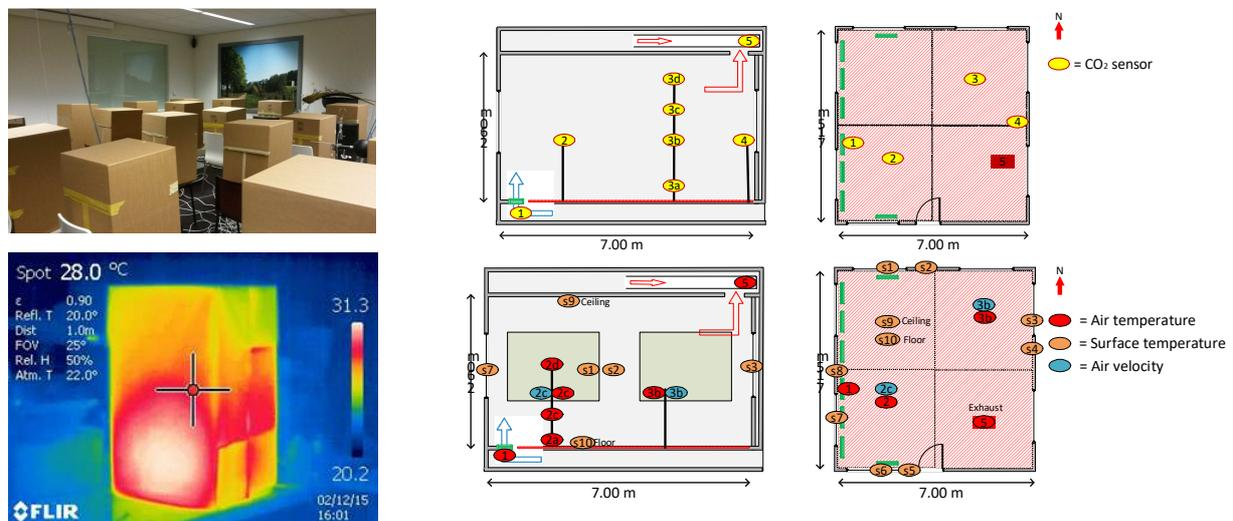
Figure 2. Photo of the full scale mock-up classroom (top-left), with heated boxes representing pupils (low-left) and measurement positions (right).
