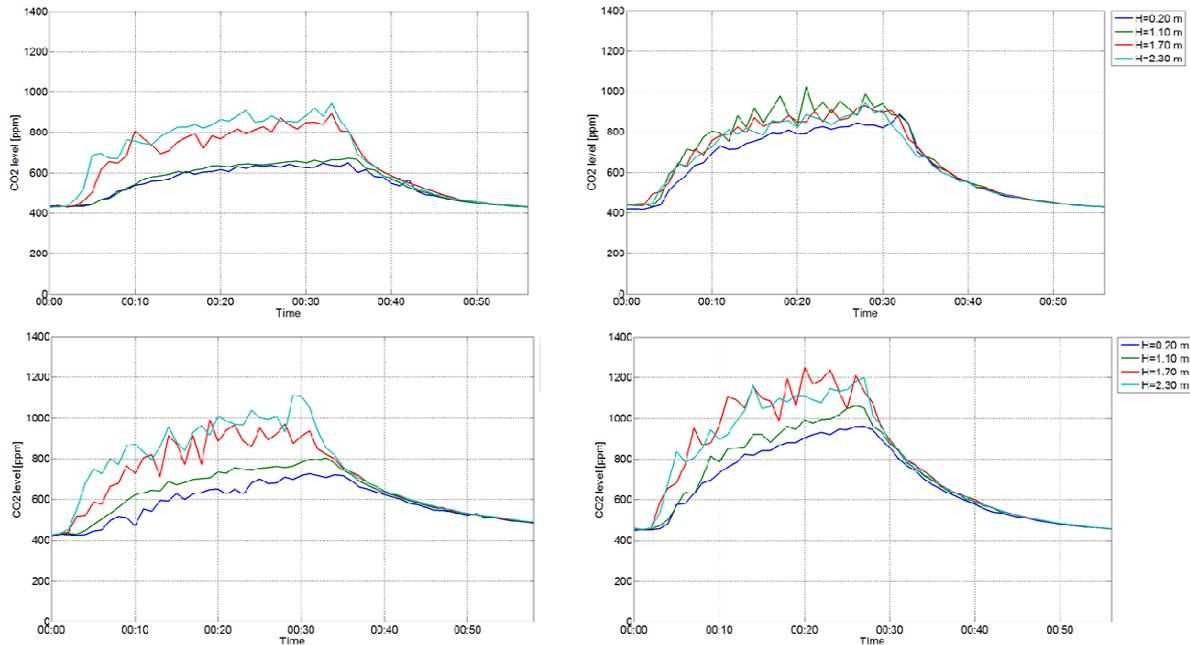
Figure 5. Continuous CO<sub>2</sub> measurements (mock-up; Top graphs at ~95 m<sup>3</sup>/h.grille, Bottom graphs at ~80 m<sup>3</sup>/h.grille; Left graphs for original system, Right graphs for mixing situation).
