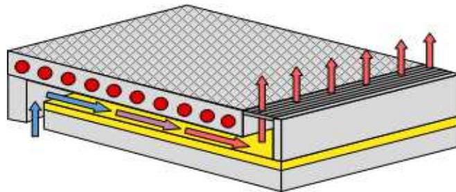
Figure 1. Schematic image of the ventilation air flow passing under the radiant floor.
