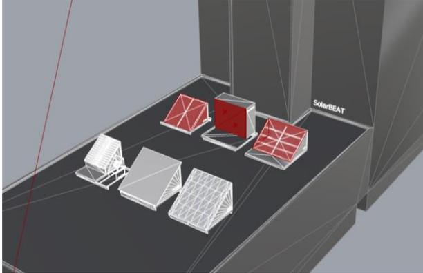
Fig. 5. Geometric representation of the SolarBEAT test set-up. The CIGS panels are located in the construction in the middle row with the red vertical façade.
