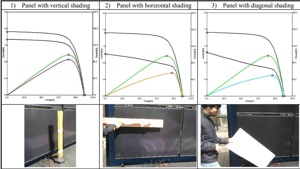
from the horizontal shading experiment, as shown by orange color. And finally the fourth situation is a combination of vertical and horizontal shading which we call diagonal shading.
