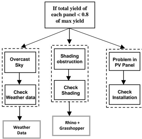
Fig. 2. Fault detection logic for installed PV
