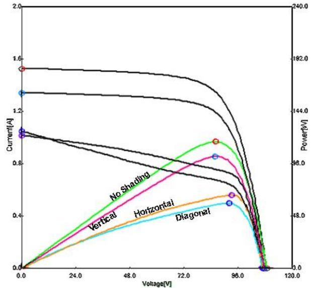
Fig. 6. Maximum power point and I-V curve for all different situations
