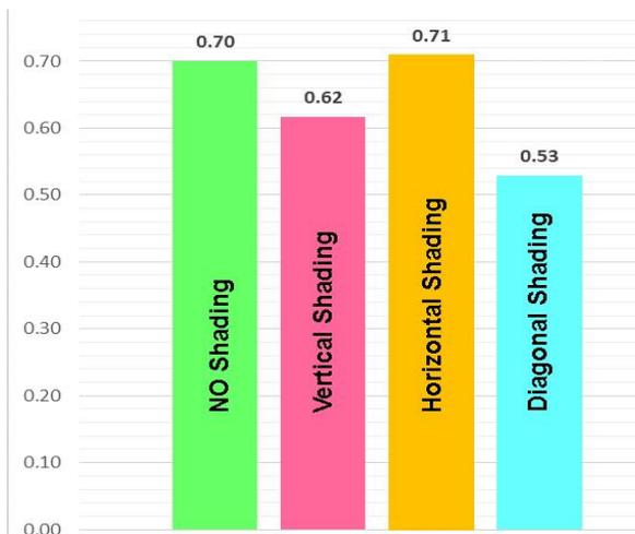
Fig. 7.Fill Factor for I-V curve of different shading situation
