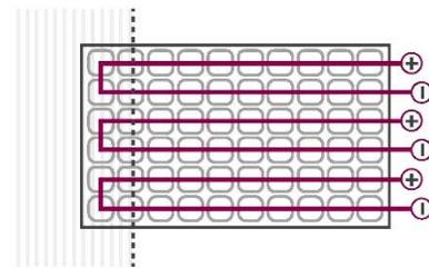
Fig. 1. The situation that shading is covering parts of the PV circuit and also will affect the output energy yield.
