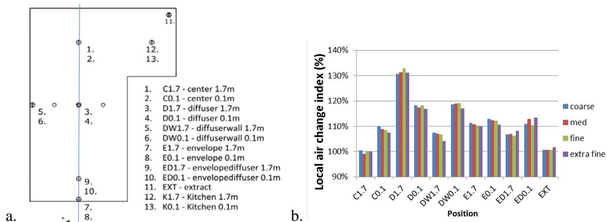
Figure 3. Room positions as used for the comparison (left); Grid sensitivity result for LACI at the room positions (right; K1.7 and K0.1 not included).
