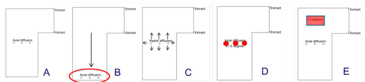
Figure 2. A. Base case, B. Envelope case, C. Radial diffuser case, D. Heating/cooling case and E. Hot patch case.
