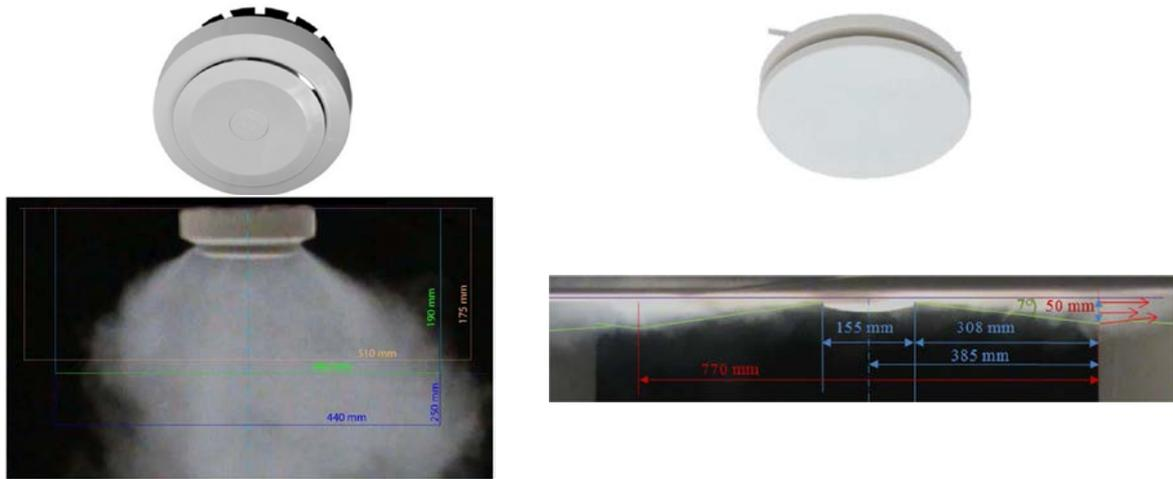
Figure 1. Axial diffuser (left), radial diffuser (right); Bottom pictures show (vertical) smoke test results.
