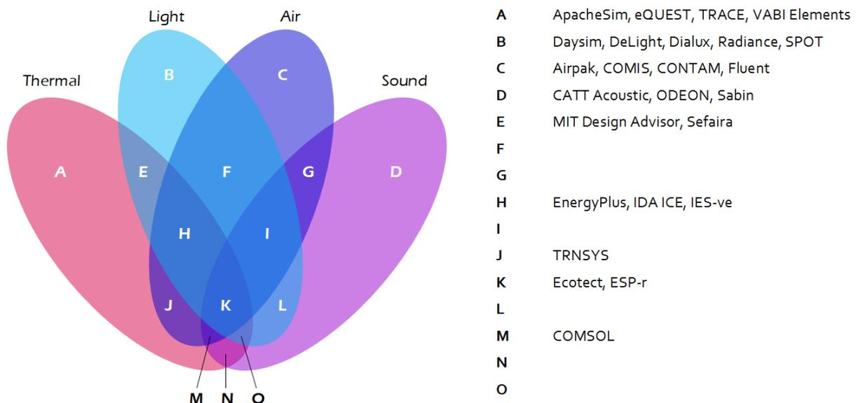
Figure 2. Coupling between physical domains in several state-of-the-art building performance simulation tools (non-exhaustive list).
