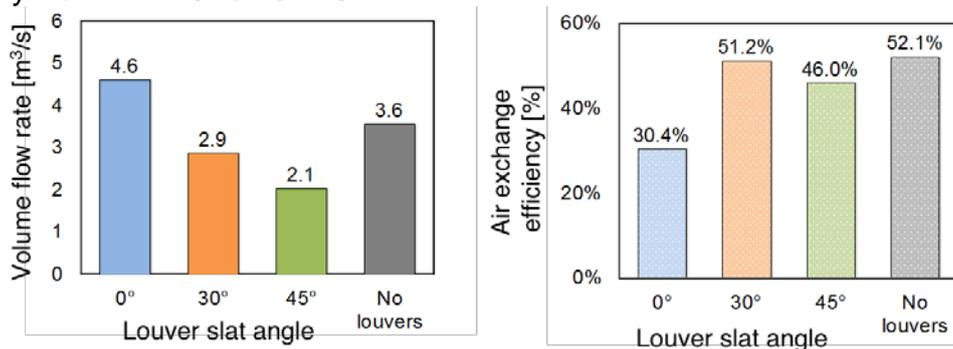
Figure 4. (a) Volume flow rates and (b) air exchange efficiency for the four different window configurations.
