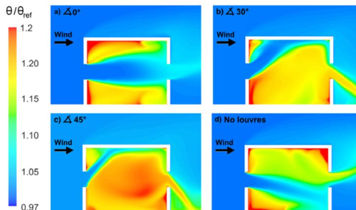
Figure 7. Contours of dimensionless temperature ( $\theta/\theta_{ref}$ ) obtained from vertical center plane around and inside the building for different louver slat angles: (a)  $0^\circ$ , (b)  $30^\circ$ , (c)  $45^\circ$ , and for (d) window without louvers.  $\theta_{ref} = 20^\circ\text{C}$ .
