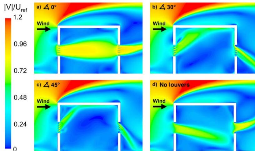
Figure 6. Contours of dimensionless velocity ( $|V|/U_{ref}$ ) in vertical center plane obtained from the non-isothermal simulations for different louver slat angles: (a)  $0^\circ$ , (b)  $30^\circ$ , (c)  $45^\circ$ , and for (d) window without louvers.  $U_{ref} = 6.97$  m/s.
