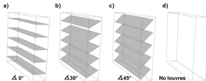
Figure 3. Window configurations studied. (a-c) Windows equipped with louvers with slat angles of: (a)  $0^\circ$ , (b)  $30^\circ$ , (c)  $45^\circ$ , and (d) without louvers.
