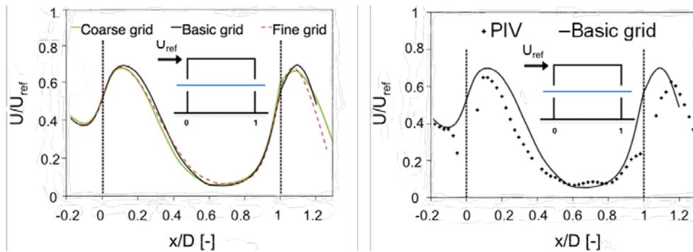
Figure 2. (a) Results of the grid-sensitivity analysis. (b) Comparison of isothermal CFD simulations using the basic grid (solid line) with PIV measurements (symbols) from Karava (2008) in terms of wind speed ratio ( $U/U_{ref}$ ) along centerline.
