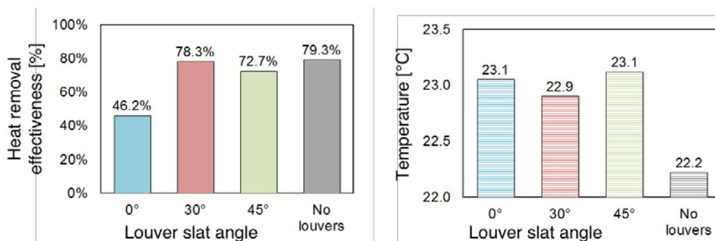
Figure 5. (a) Heat removal effectiveness; (b) average indoor temperature ( $\theta_{ref} = 20^\circ\text{C}$ ) for the four different window configurations.
