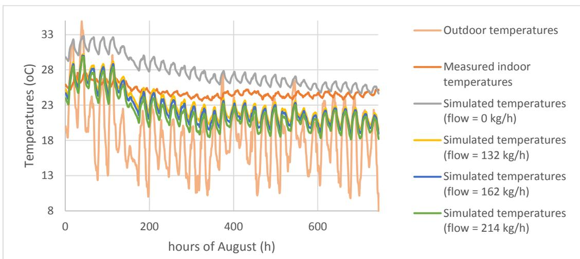
Fig. 4. Impact of increased air flows rates on the temperatures of the living room during August
