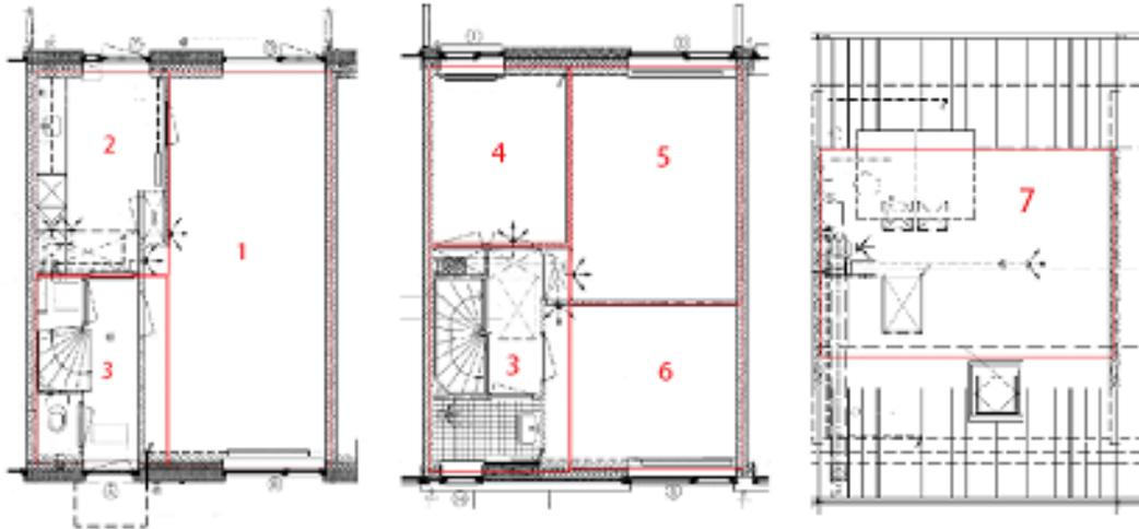
Figure 1. Plant of modelled passive house a) Ground floor: zone 1 – living room; zone 2 – kitchen; zone 3 – bathroom + hall; b) First floor: zone 3 – bathroom + hall; zones 4, 5 and 6 – bedrooms; c) Second floor: zone 7 – attic
