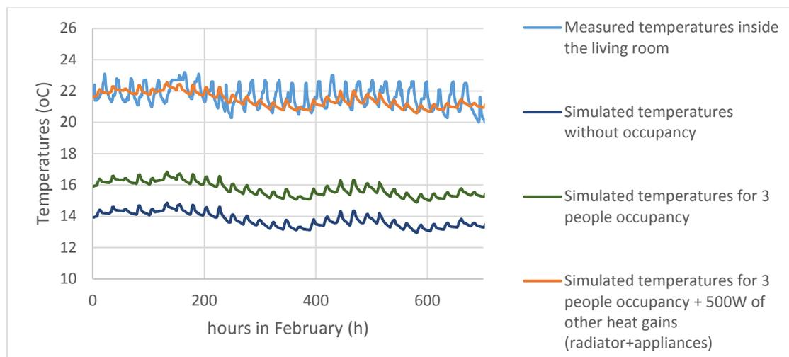
Figure 3. Measured and simulated temperatures inside the living room of the studied passive house during February for flow rate 132 kg/h of pre-heated outdoor air
