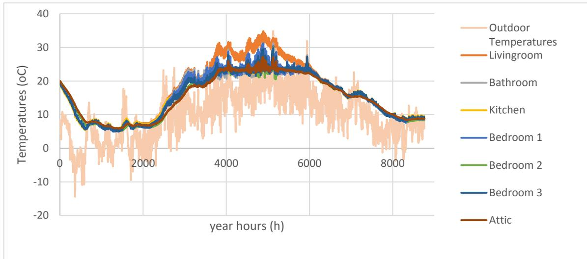
Figure 2. Simulated indoor temperatures for studied renovated passive house
