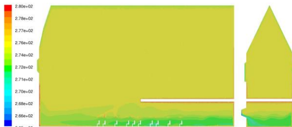
Figure 8 – Temperature field, case with 65 visitors (contours of temperature [K])
