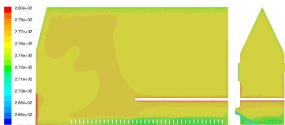
Figure 9 – Temperature field, case with 304 visitors (contours of temperature [K])
