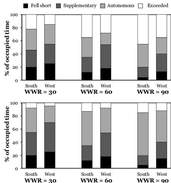
Figure 3. Useful daylight illuminance results for the regular window (top) and switchable VLT window (bottom). Results are shown for two façade orientations and three window-to-wall ratios.
