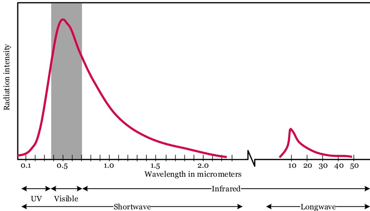
Figure 1. Illustration comparing the intensity of solar and terrestrial radiation. Because of the sun's high surface temperature, most of its energy is radiated at wavelengths shorter than  $4 \mu\text{m}$ , with the greatest concentration in the visible range of the electromagnetic spectrum.
