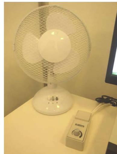
Fig. 4. Fan with control unit (gray unit in lower right, with rotary switch). Note that the regular '0-1-2' button on the fan itself was fixed in the '2' (maximum) position during the experiments.
