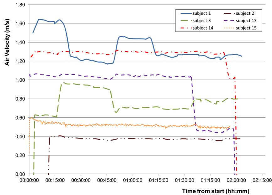
**Fig. 6.** Verification measurement outcomes for one subject that used fan no. 1: comparing the air velocity profile of this subject for session B (created by the research team) with that of session A (original velocity profile as created by this subject).
