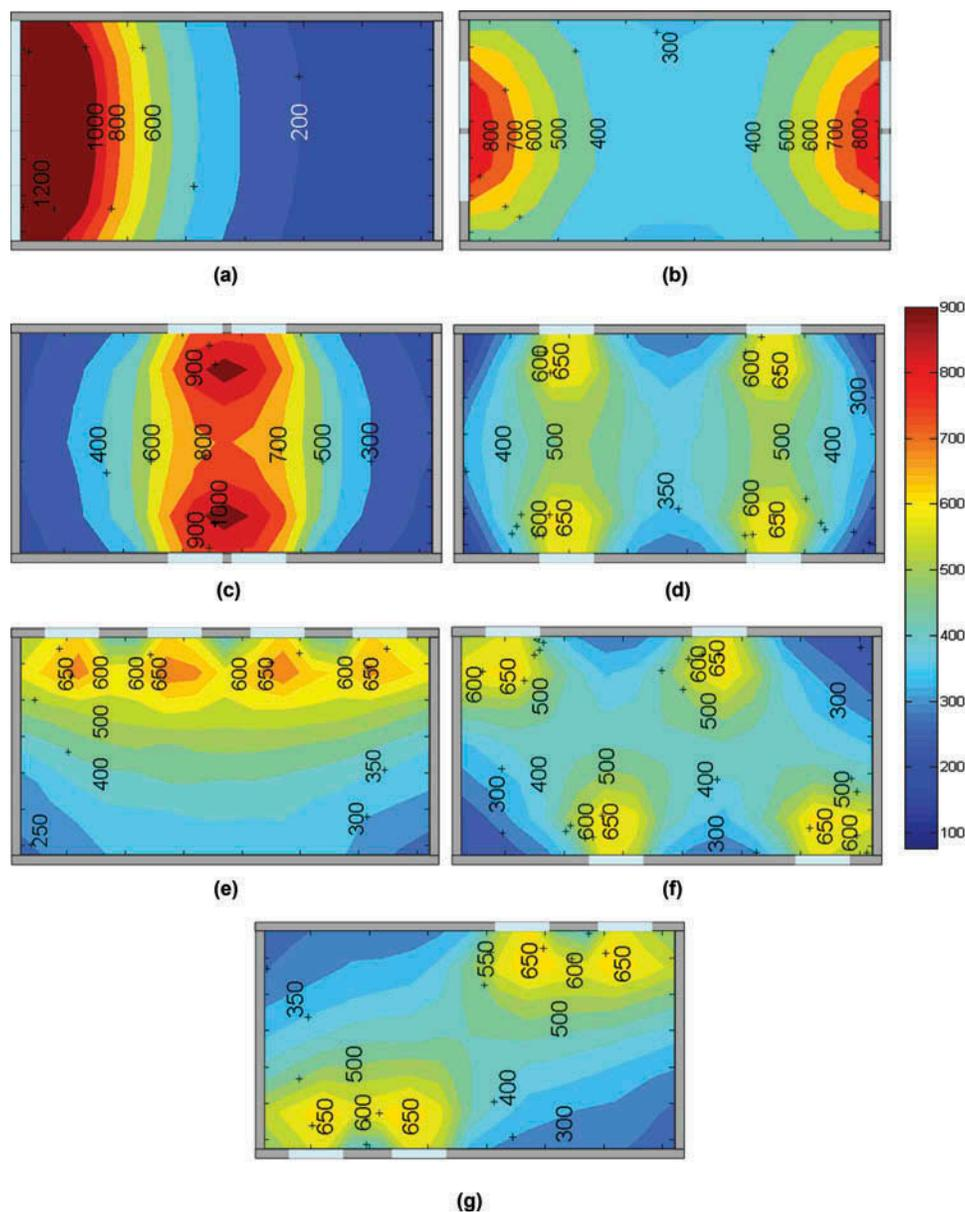
**Fig. 10** False color maps of the simulated horizontal illuminance ( $lx$ ) under configurations (a) 1, (b) 2, (c) 3, (d) 4, (e) 5, (f) 6, and (g) 7.
