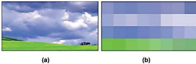
**Fig. 2** (a) Original displayed view and (b) displayed view after applying a mosaic filter.
