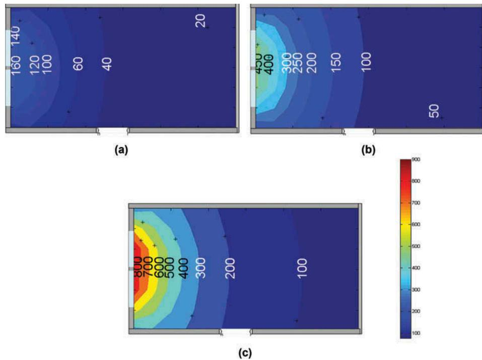
**Fig. 7** False color maps of the measured workplane illuminance (lx) under (a) 25%, (b) 62.5%, and (c) 100% of the maximum setting.
