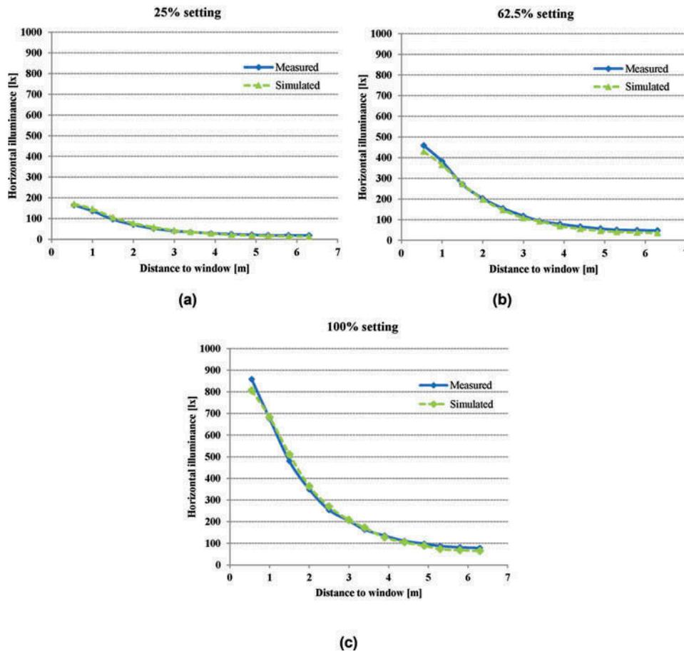
**Fig. 8** Graphs showing the relationship between horizontal illuminance at the central line on the workplane and distance to windows under the (a) 25%, (b) 62.5%, and (c) 100% of the maximum setting.
