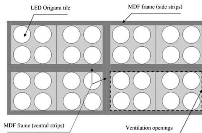
**Fig. 1** Rearview illustration of the 2  $\times$  4 Origami BPG762 arrays in the prototype.
