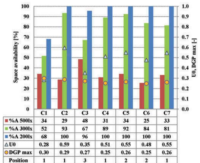
**Fig. 9** Graphs showing the relationship between space availability, uniformity, and maximum DGP in the test room under the simulated configuration scenes.
