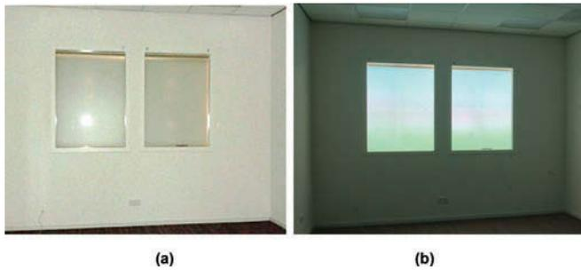
**Fig. 3** Prototype appearance from inside the test room at (a) off and (b) on conditions.
