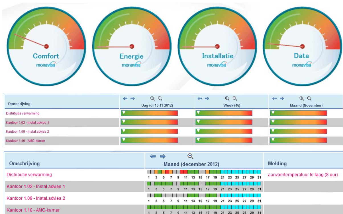
Figure 1. Monavisa interface and different levels of detail at which Monavisa shows information. From top to bottom: general overview for each category [Comfort, Energy, Building systems, Data availability]; overview for daily, weekly and monthly performance for each monitored room; detailed overview and assessment for each time interval and notifications for each monitored room [monavisa.dwa.nl].
