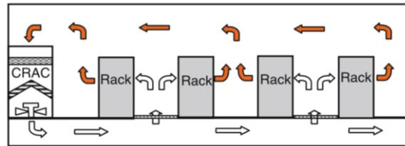
Fig. 3 – Conventional DC arrangement with under-floor plenum [7]
