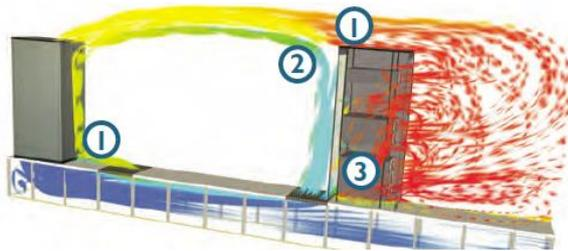
Fig. 2 – Common DC Air-Flow Imperfections [6] (1 – Reverse flow; 2 – Bypass; 3 – Recirculation)
