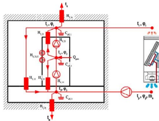
Fig. 5 - Scheme of Server Room Model
