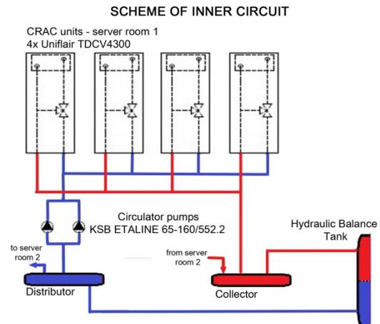
Fig. 1 - Scheme of cooling system, inner circuit
