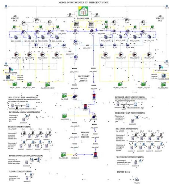
Fig. 4 – Numerical Model in TRNSYS software
