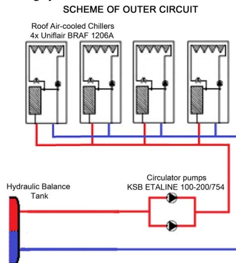
Fig. 2 - Scheme of Cooling System, Outer Circuit
