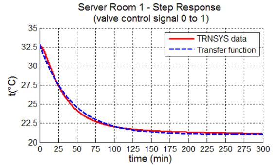
Fig. 6- Step Response of Supply Air Temperature
