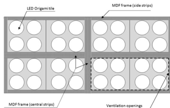
**Figure 1.** Rear view illustration of the 2 × 4 Origami BPG762 arrays in the prototype; taken from Mangkuto et al. (2014)
