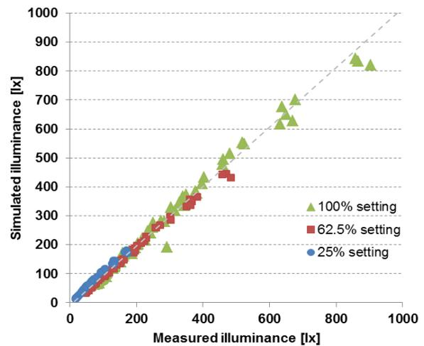
**Figure 5.** Graphs showing the relationship between simulated and measured horizontal illuminance under 25%, 62.5%, and 100% of the maximum setting
