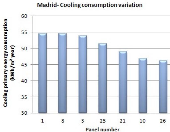
Figure 7 Variation of cooling consumption due to TSR variation of HPL
