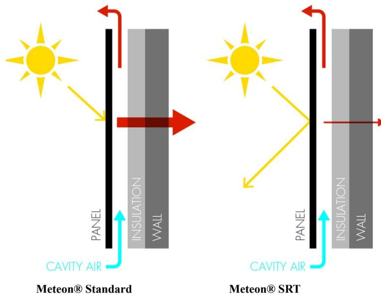
Figure 6 Energy balance in opaque facade part with Trespa® Meteon® SRT panels
