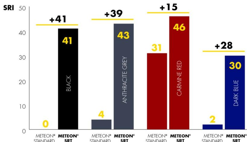
Figure 5 SRI difference between Meeon® Standard and Meeon® SRI
