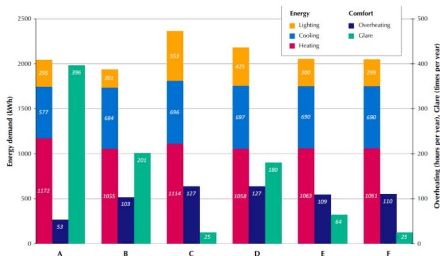
Figure 2 Results of the exploratory simulation study in terms of energy consumption and comfort. Cases A is a reference case with external solar shading. Cases B-F represent different window control strategies (Loonen et al. 2010).
