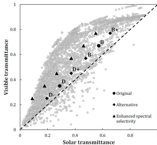
Figure 3 Overview of window properties showing dark (D) and bright (B) states. Triangles indicate window options with enhance spectral selectivity.
