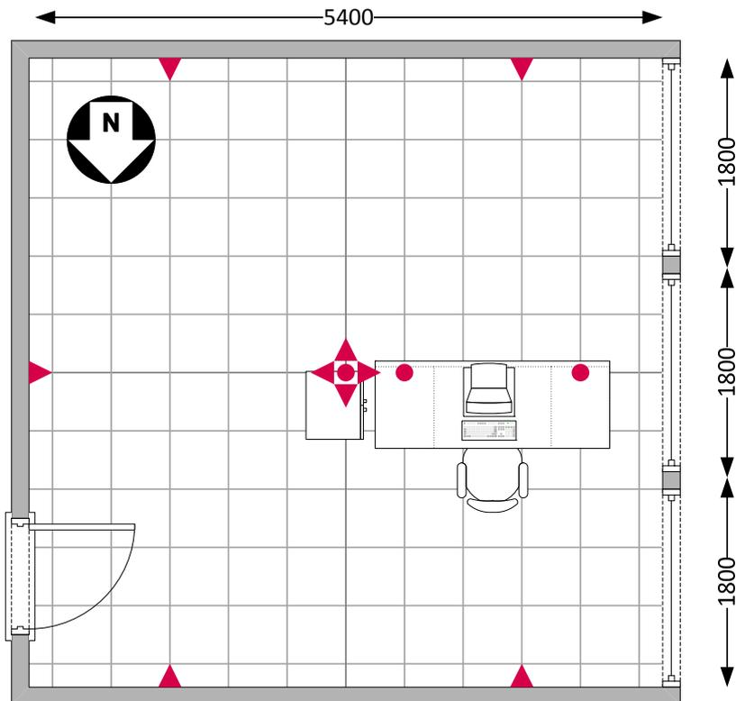
**Figure 2:** Floor plan of the test room, with the positions and direction of the computer screen relative to the facade. Red triangles indicate horizontal illuminance sensors; red dots indicate vertical illuminance sensors.
