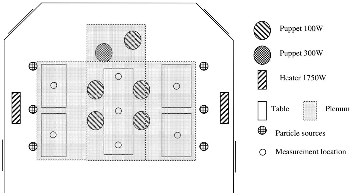
Figure 1. Floor plan of the experimental setup.
