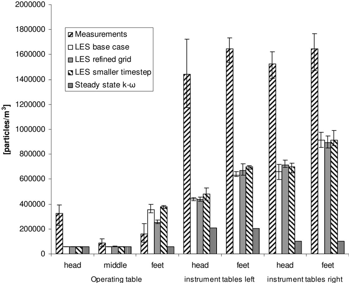
Figure 2. Particle concentrations from measurements and simulations. Values indicate the average from four measured values; error bars indicate the minimum and maximum values in these.
