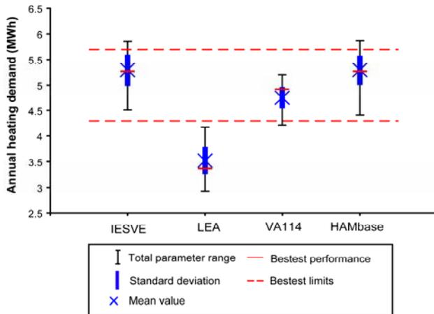
Figure2, Tool performance comparison - Annual heating demand [MWh]
