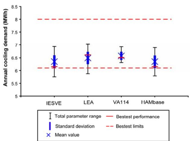
Figure3, Tool performance comparison - Annual cooling demand [MWh]
