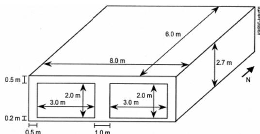
Figure 1. Bestest Case 600 - Geometry
