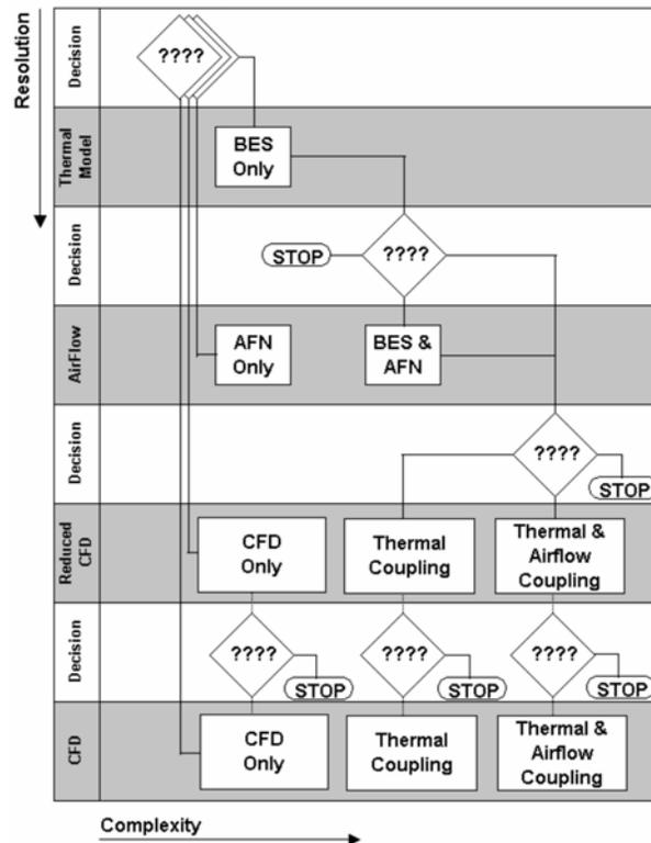
Figure 1. Prototype airflow based Coupling Procedure Decision Methodology.
