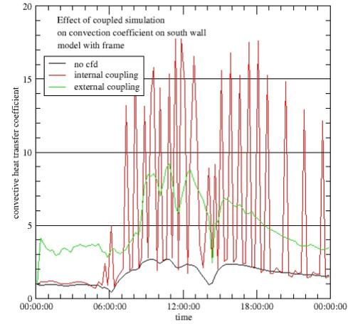
Figure 8. CHTC of south wall (simplified model) Figure 9. CHTC of south wall (model with frame)
