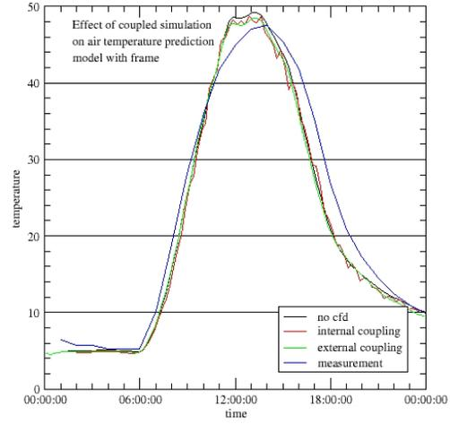
Figure 6. Air temperature comparison (simplified model) Figure 7. Air temperature comparison (model with frame)
