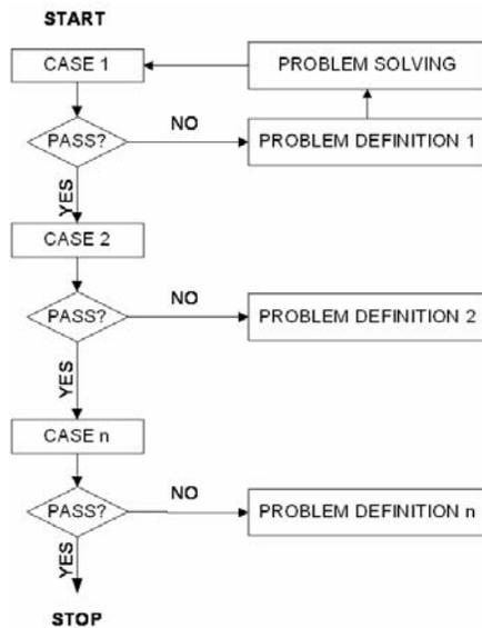
Figure 9: Validation methodology with BESTEST
