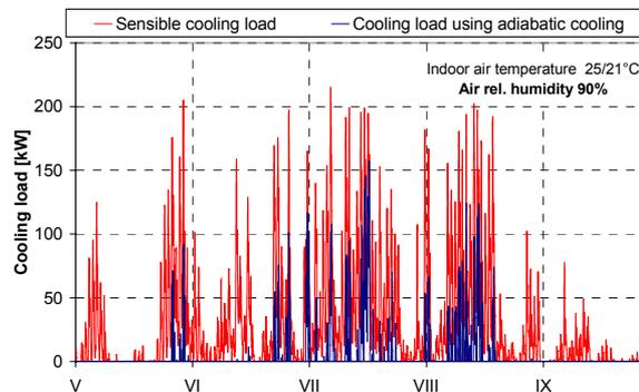
Figure 10: Reduction of the cooling load due to direct evaporative (adiabatic) cooling
