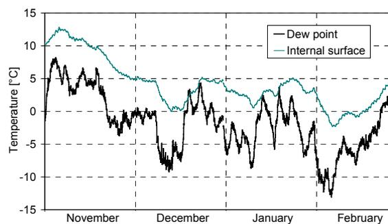
Figure 6: Internal surface temperature on the north wall and dew point temperature
