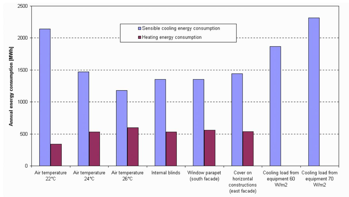
Figure 3: Comparison of different design concepts with respect to energy consumption
