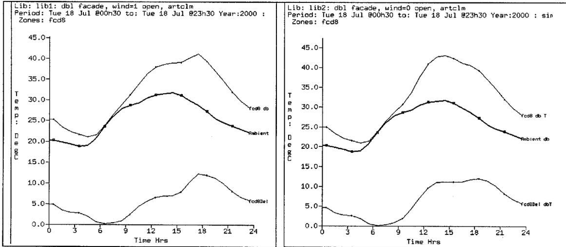
**Figure 4** Predicted air temperatures in the double-skin façade during one of the warmest summer days in Prague. Upper lines represent outlet temperatures. Middle lines represent inlet temperatures (ambient). Lower lines represent the temperature rise in the façade. The left graph corresponds to the final design of the double-skin façade with wind forces taken into account. The right graph represents the same situation without taking into account the airflow driving forces due to wind.
