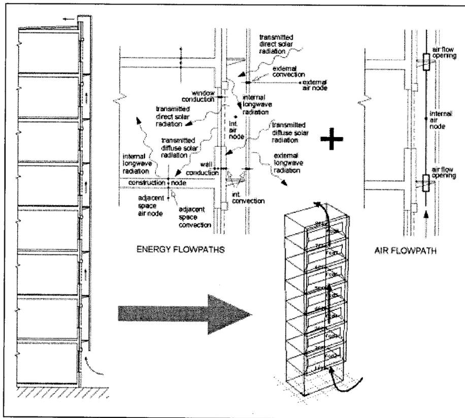
**Figure 3** The model of the double-skin façade. On the left: cross section of the double-skin façade system. Above: schematic representation of the super-imposed thermal and airflow network models. Bottom: graphic feedback from the simulation environment.
