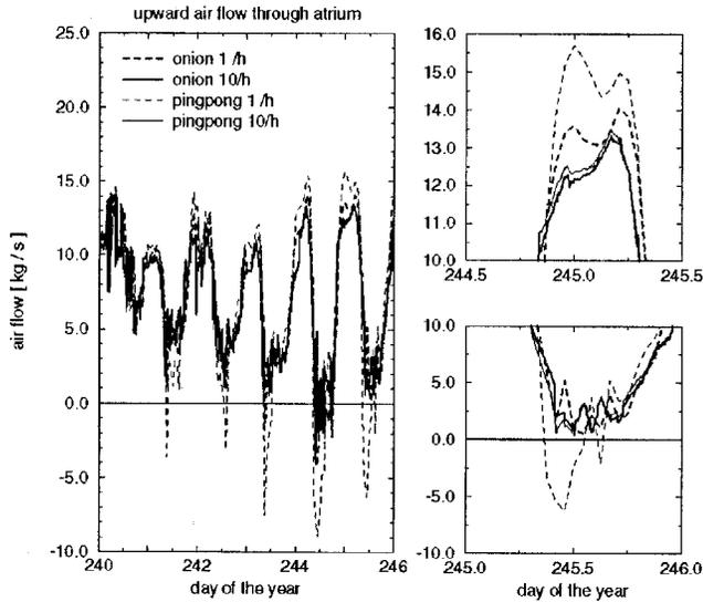
**Figure 2** Typical airflow variations in a natural ventilated glazed vertical building structure, such as a double-skin façade. Graphs on the right show different coupled and decoupled solutions for temperature and airflow (Hensen 1999b).
