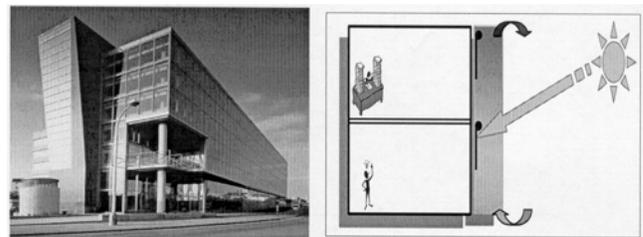
**Figure 1** Typical example and principle of double-skin façade.
