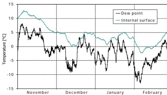
Figure 6: Internal surface temperature on the north wall and dew point temperature during the winter period
