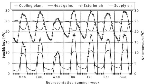
Figure 3: Optimized operation of air-conditioning system (indoor air temperature set point is 26 °C)
