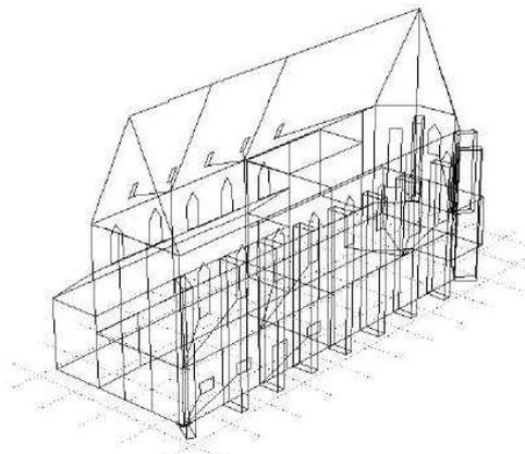
Figure 4: ESP-r model of the building
