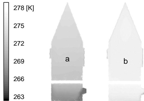
Figure 8: Air temperature distribution in the transversal section for cases with (a) open and (b) closed roof windows
