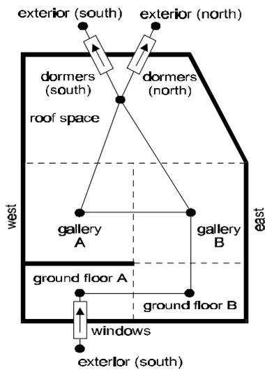
Figure 5: Diagram of thermal zones and airflow network
