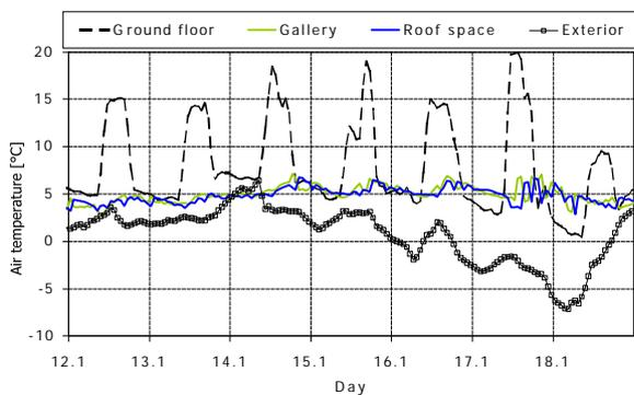
Figure 7: Air temperatures during a typical winter week
