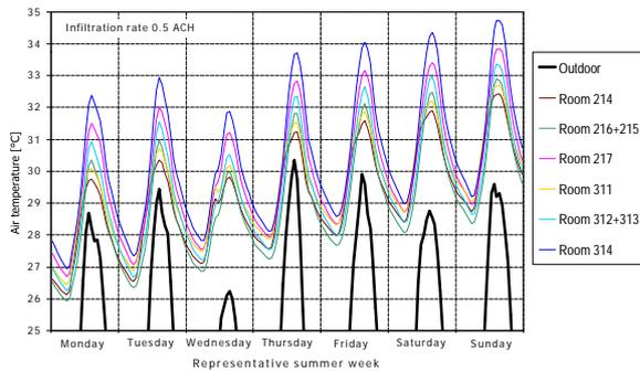
Figure 2: Temperatures of indoor and outdoor air (ventilation without air-conditioning)
