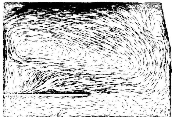
Figure 9: Air velocity field in the central longitudinal section for the case with closed roof windows (max. velocity 0.6 m/s).
