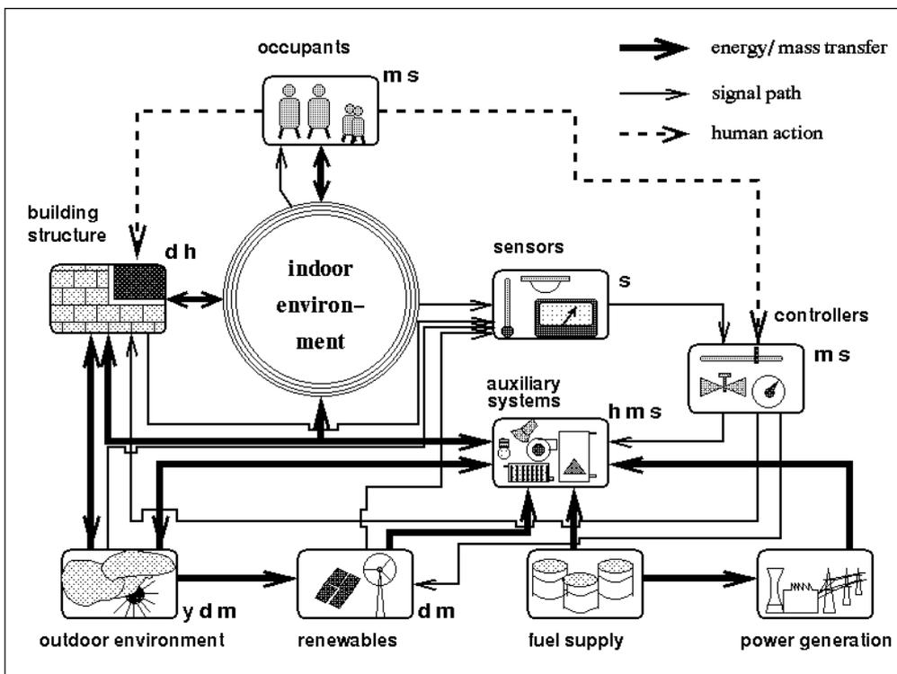
Figure 2 : Schematic overview of research field: the building as an integration of energy systems
